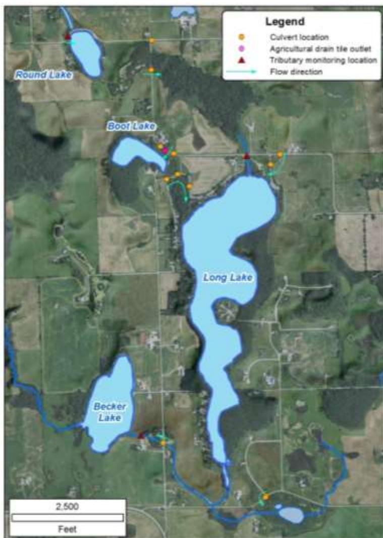
**Figure 3.2-10. Aerial photo showing study lakes and stream monitoring sites.** The three triangles are the sites of the continuous recorders. The culvert sites were sampled when flow occurred.
