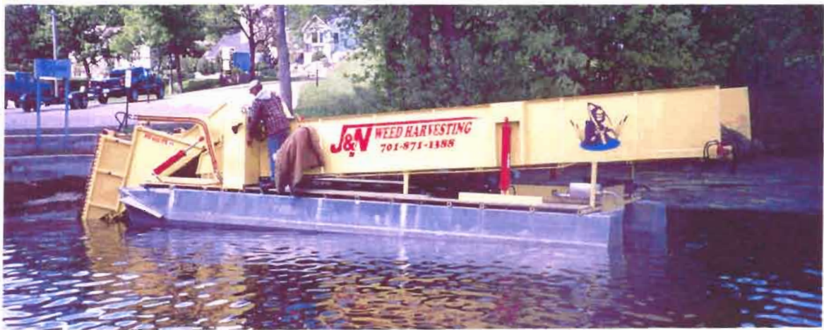
Figure 30. A mechanical harvester is recommended for picking up fern pondweed in the shallow southwest bay if plant management is considered.
