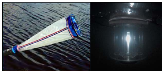
Ichthyoplankton tow nets (left) and light traps (right) were set overnight to catch larval fish.
