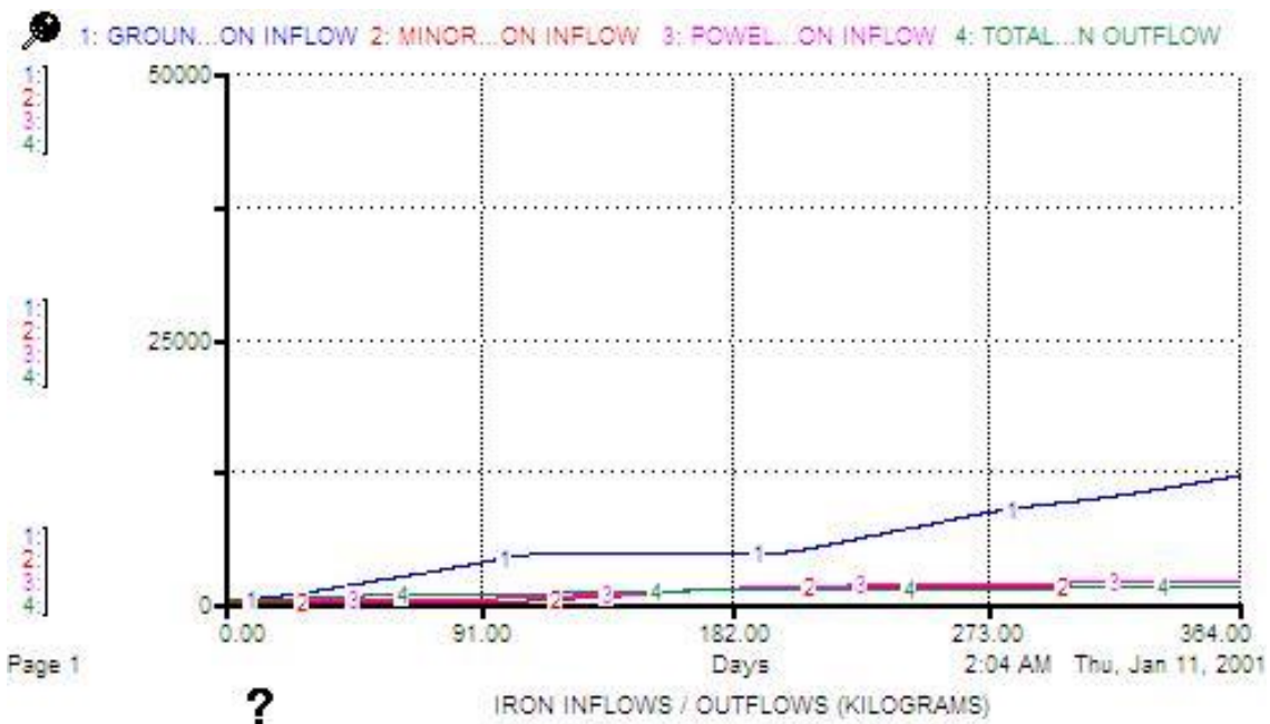
STELLA GRAPH 4. This graph models the difference from GRAPH 3 with a 1 foot increase in the elevation of the Dead Pike Lake outlet stream and a wetland biofilter system in Powell Marsh. The Blue line (#1) represents the iron groundwater load. The Red line (#2) represents the iron load from Pete's and Deerfoot Marsh creeks. The Purple line (#3) represents the iron load from Powell Marsh. The Green Line (#4) represents the iron load leaving Dead Pike Lake.
