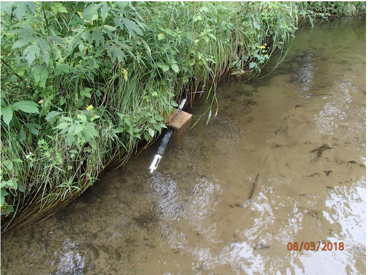
Photo 4: Continuous Dissolved Oxygen and Temperature Meter Deployment at Davies Creek at County K in 2018. Photo taken by D. Bolha on August 3 rd , 2018.
