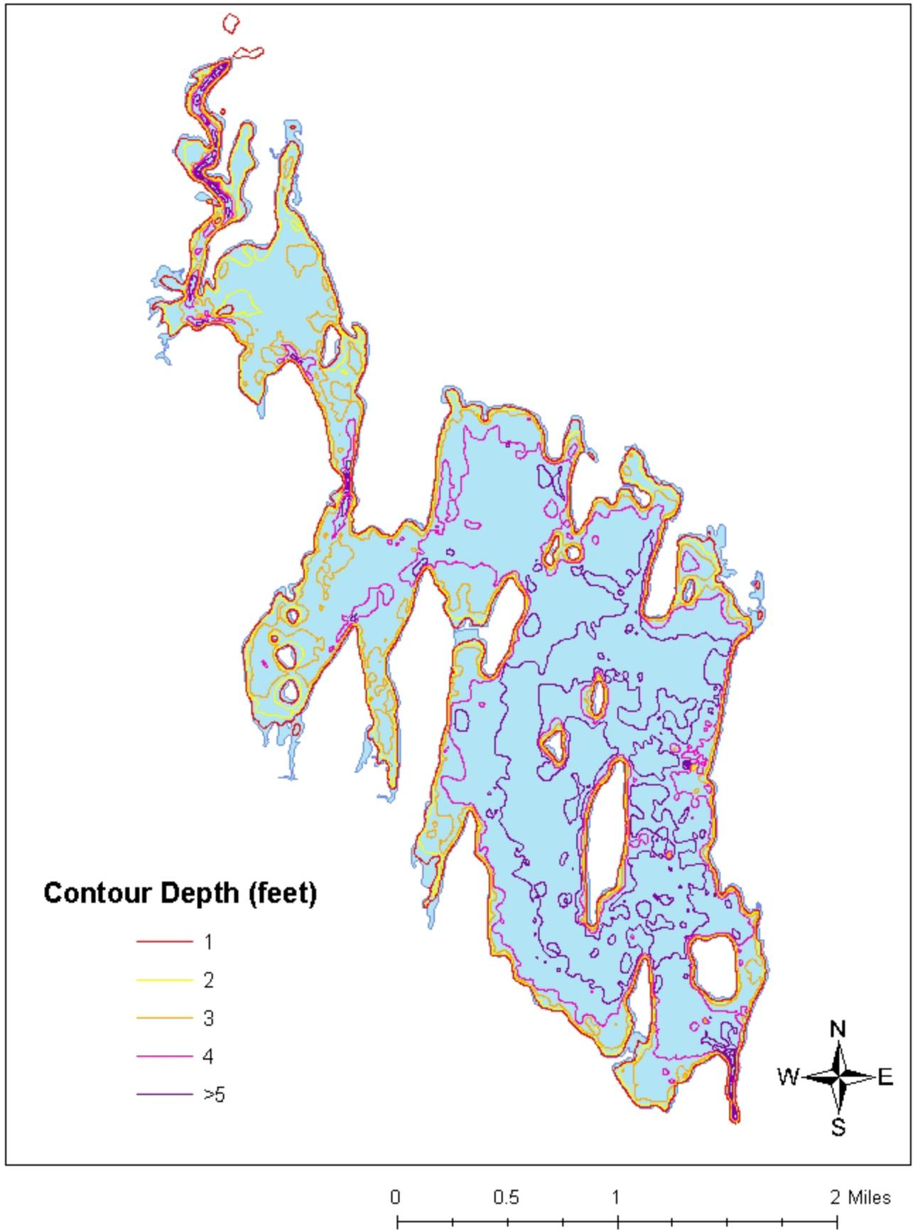
Figure 3. Lake Sinissippi Bathymetric Contours
