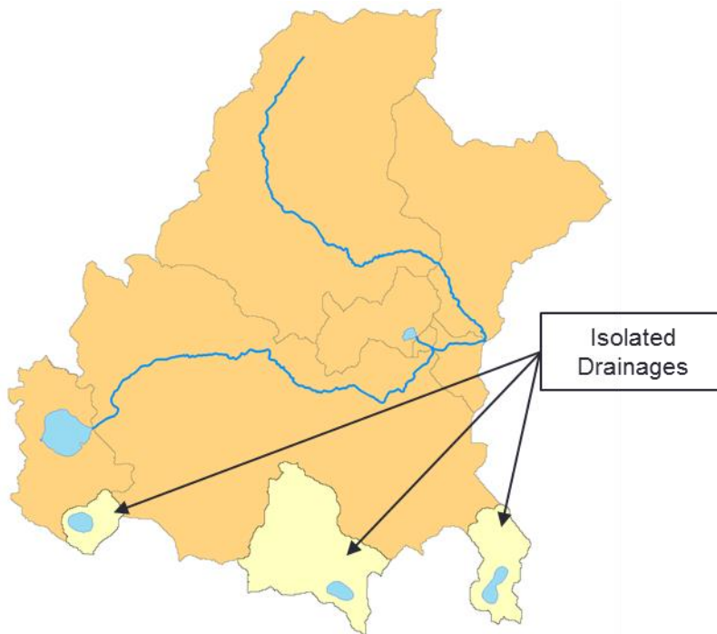
Figure 2. Example of isolated drainage areas in the WDNR 1:24,000 hydrography geodatabase. Isolated drainage areas were used to estimate internally drained areas in SWAT subwatersheds.
