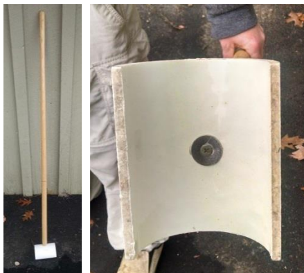
Wood Calibration Stick – a 6 inch length of 4 inch inner diameter PVC pipe cut in half lengthwise attached perpendicular to a 5 foot long pole that is used to measure large wood in the water. One foot intervals should also be marked on the stick (to measure 2-foot depth).
