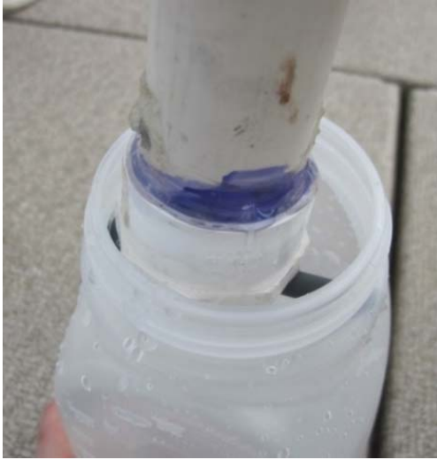
Photo 2. Emptying the water sample from the integrated sampler device into the custom mixing bottle.
