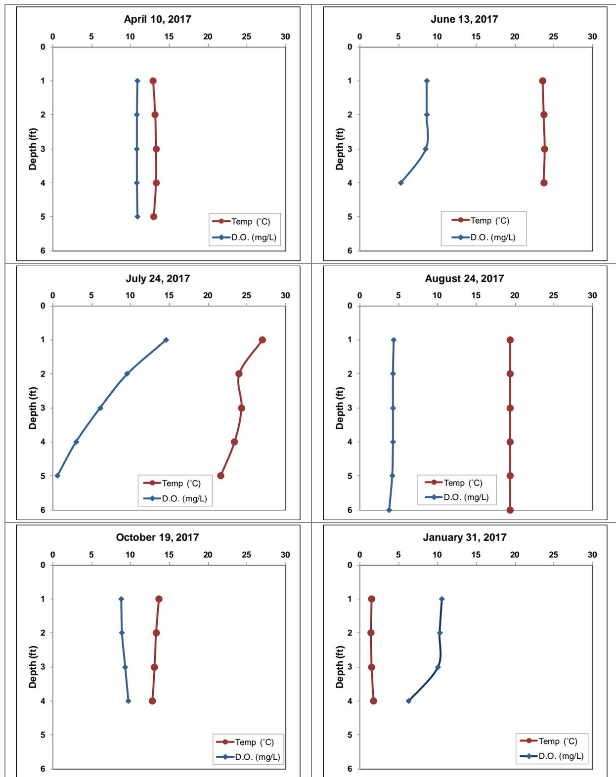
Figure 3.1-6. Lake Iola dissolved oxygen and temperature profiles.
