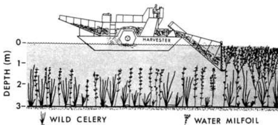
Figure 37: How a Harvester Works (Engle, 1987)
