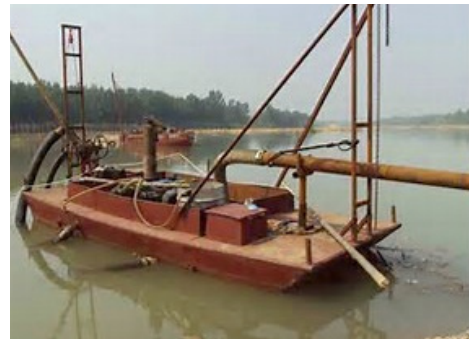
Hydraulic dredges, act like a giant floating vacuum, removing sediment.
