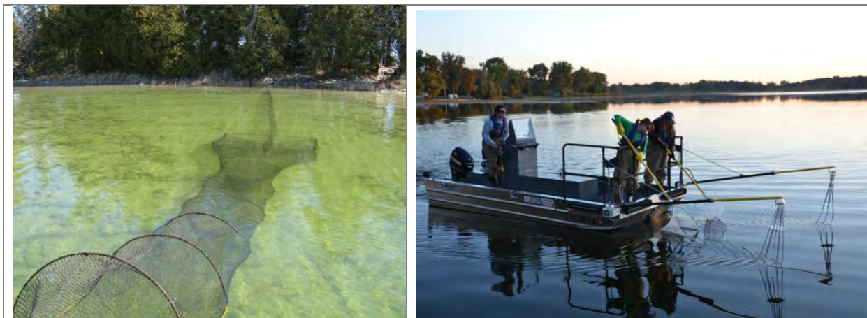
Photograph 8.1.6-1. Fyke net positioned in the littoral zone of a Wisconsin Lake (left) and an electroshocking boat (right).
