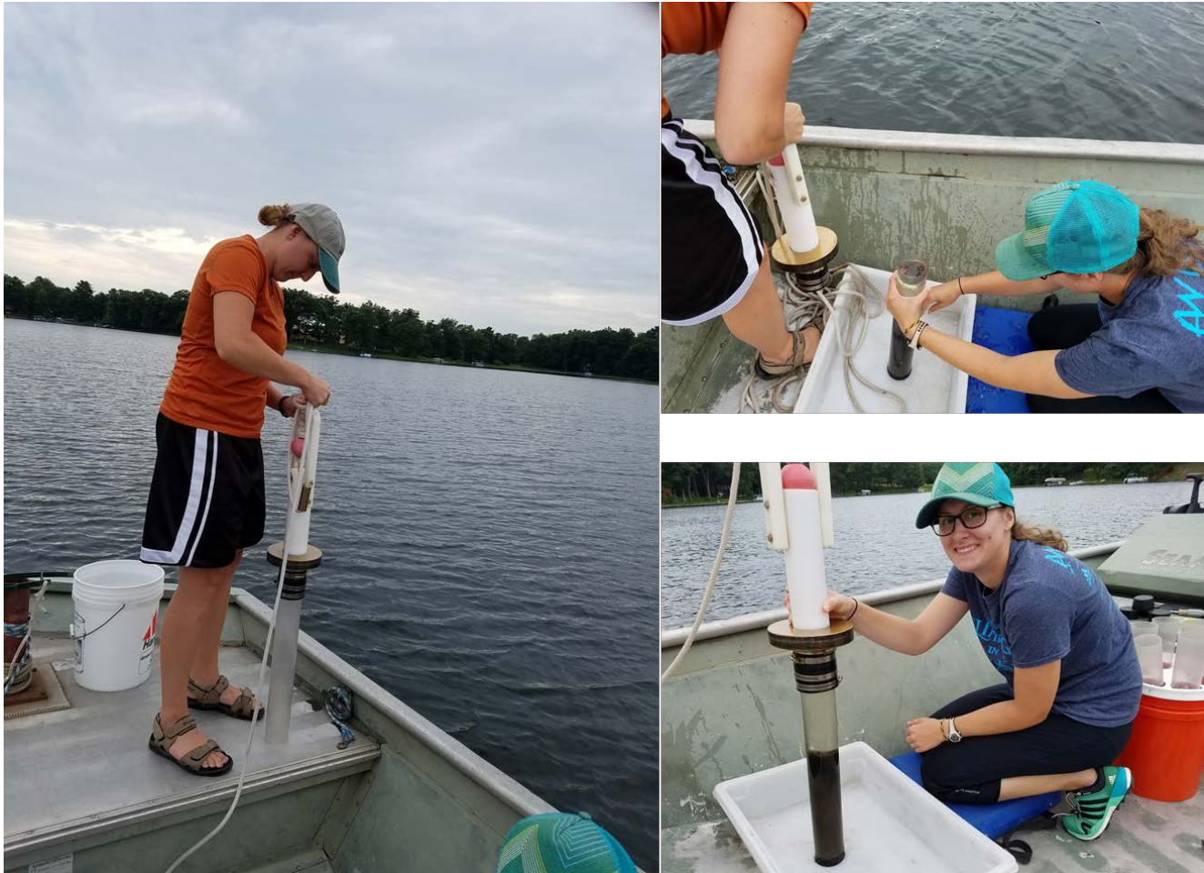
Figure 2. Sediment core apparatus and sediment coring on Horseshoe Lake.
