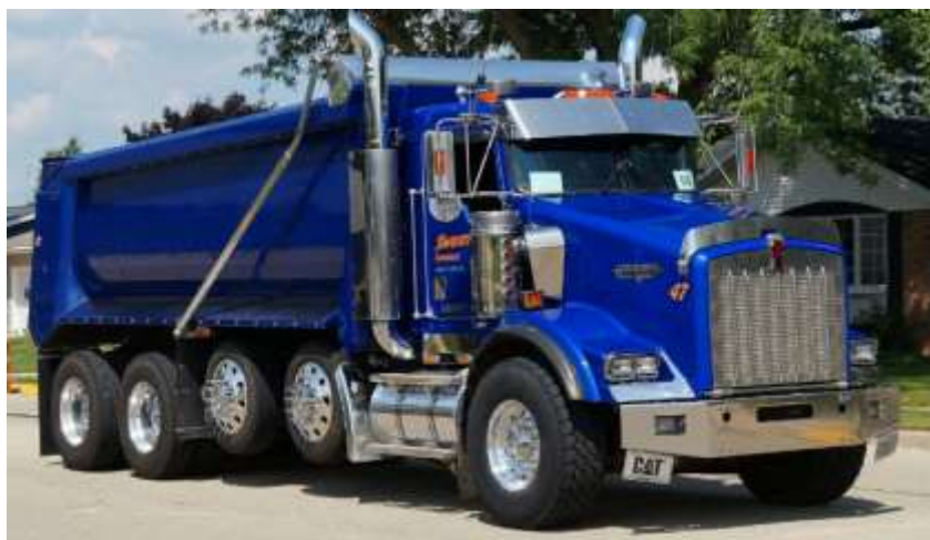
Figure 14: Quad-axle dump truck like what is used for hauling frac sand
