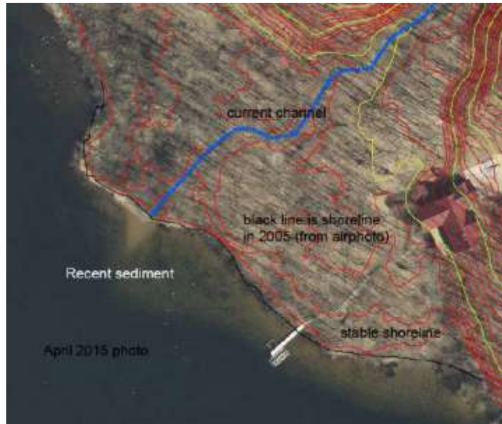
Figure 2: 2015 evidence of new sediment in the lake from the NE Wash
