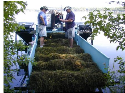
A load of cut weeds is being inspected on the weed harvester by two employees of the Lake District.
