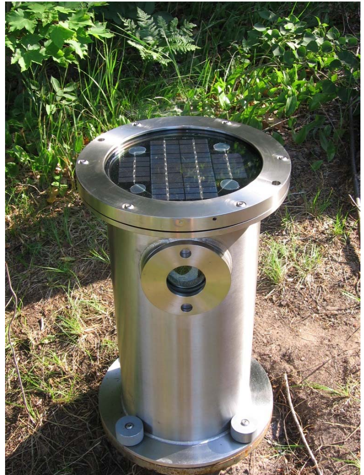
I-LIDS installed on footing
