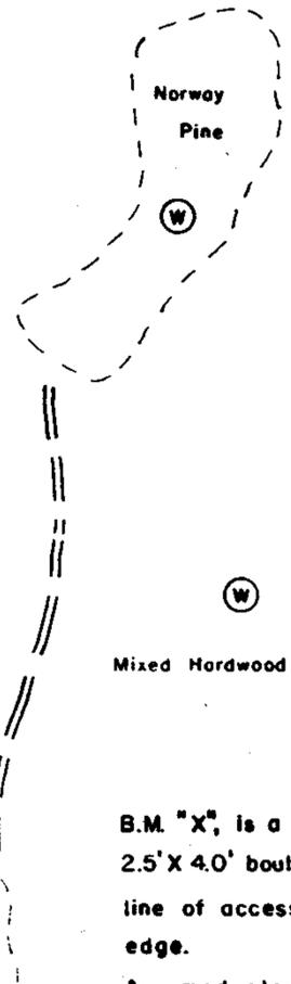
B.M. "X", is a 3" sq. cut in the top of a 2.5' X 4.0' boulder located 20' N. of center-line of access road and 87' W. of waters edge.
