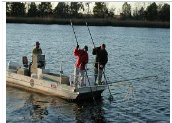
Photograph 3.6-2. Electroshocking boat (Photo from South Carolina Department of Natural Resources, SCDNR 2011)
