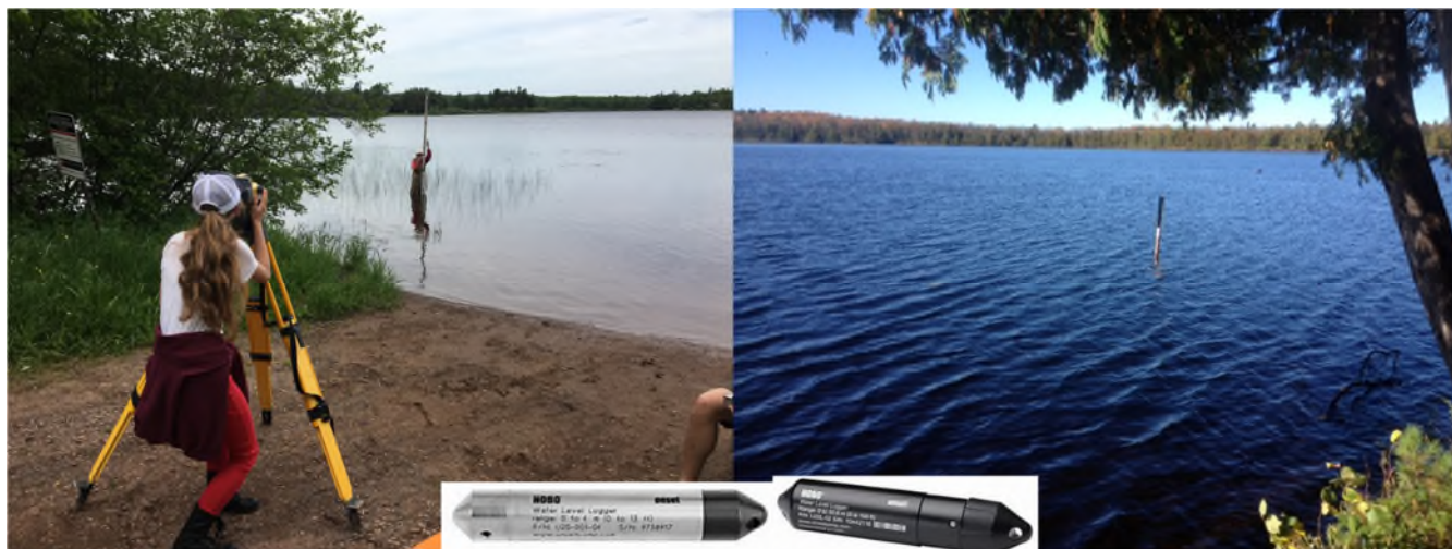
Figure E.1. Survey work to establish water level elevations (left), typical water level logger installation at the Penokee Lakes (right), and HOB0 water level loggers used in the study (middle pictures).
