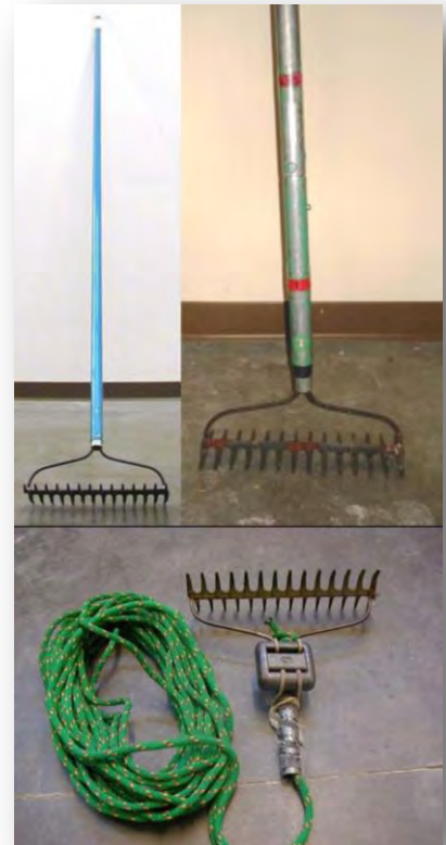
Standard PI rake: a double-headed garden rake, constructed by cutting one handle off and fixing the two heads together. Rake on a rope used for deep sites. Photo: WDNR
