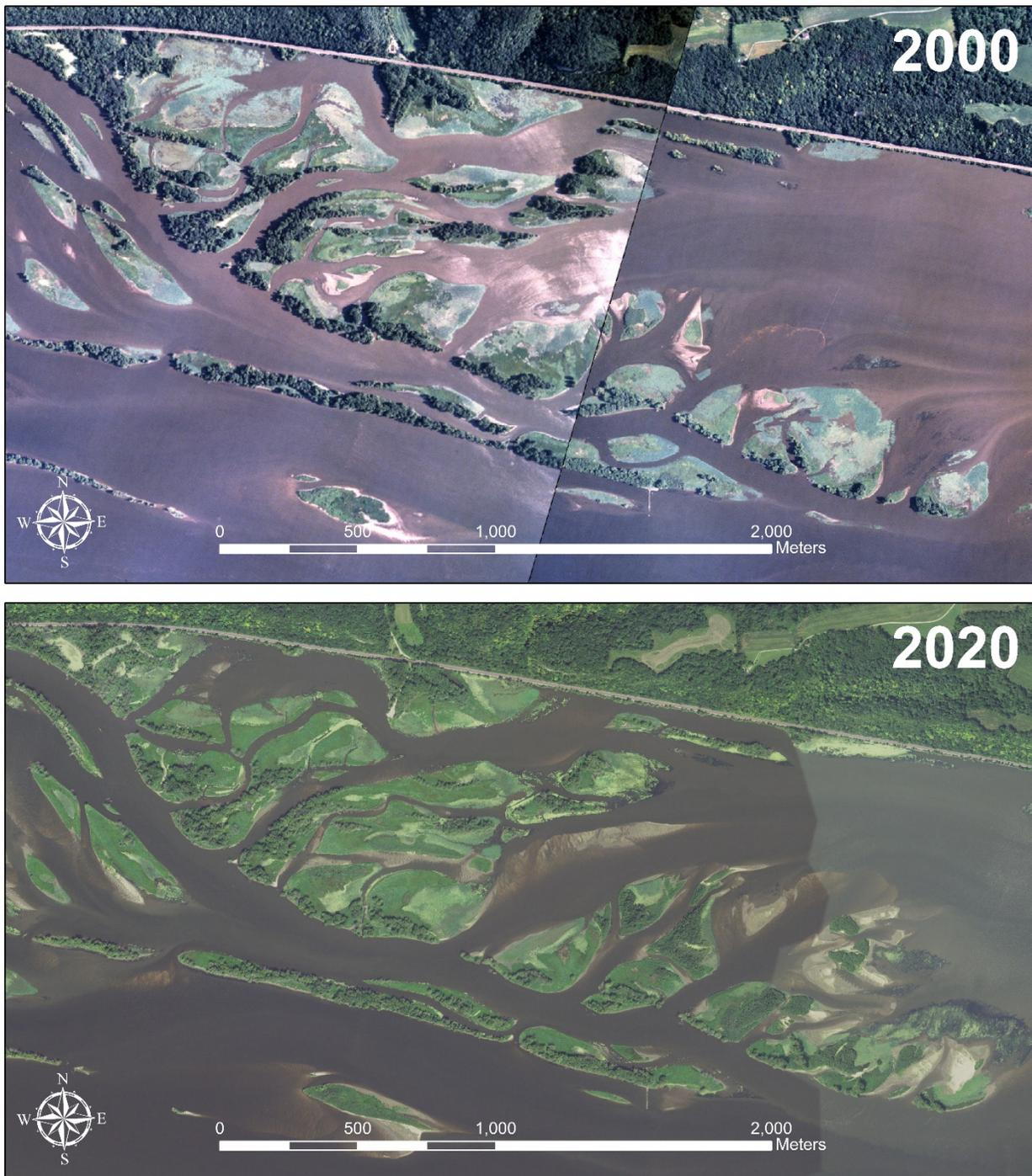
*Figure 6: Snyder Slough in Pool 11 in 2000 and 2020. Consequences of climate change such as off-channel sedimentation, loss of aquatic area and forest loss are evident over the twenty-year period. Image: Jeff Janvrin, WI DNR.*
