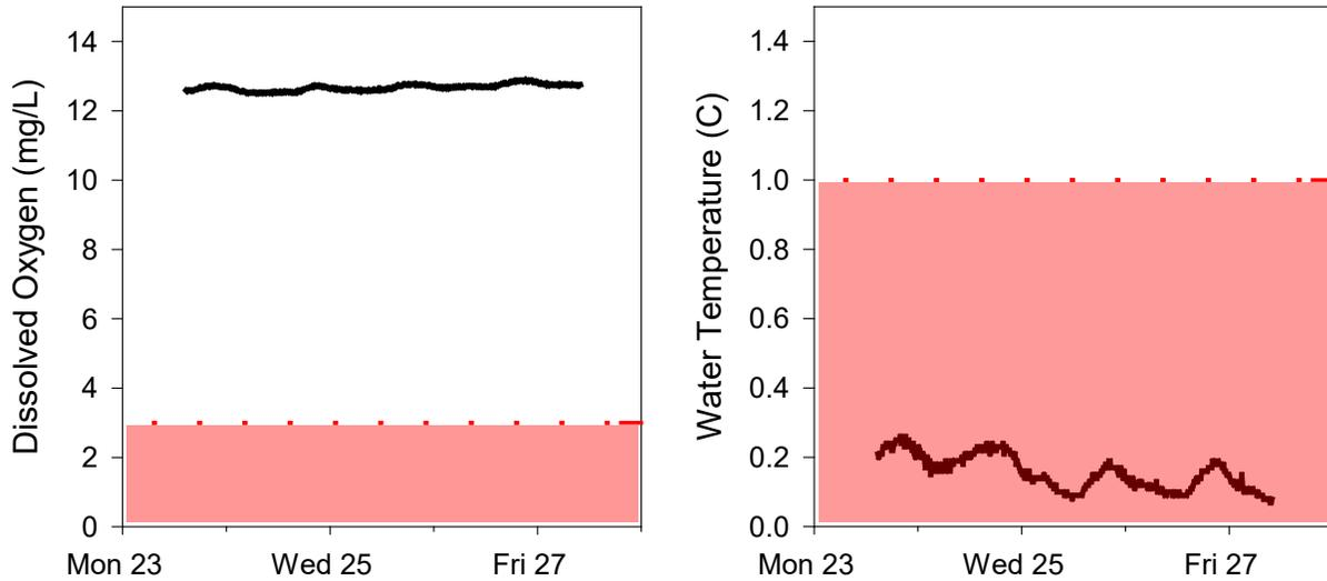
Figure 14: Dissolved oxygen and water temperature collected using continuous meters deployed under the ice in Probst Lake during a recent high discharge winter. Cold water temperature observed (< 1° C) was more indicative of a flowing channel condition than backwater condition during the winter months. The pink shading represents the poor winter habitat quality range.
