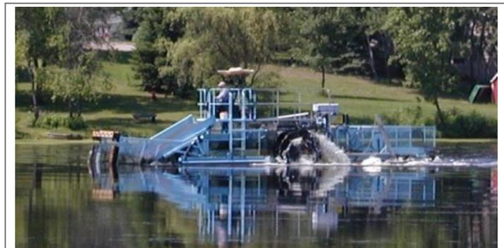
**Photograph 3.5-3. Mechanical harvester.**
