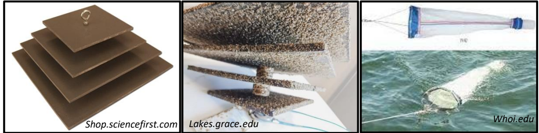
Sample plate WITHOUT zebra mussels Sample plate WITH zebra mussels Plankton tow net for veligers
