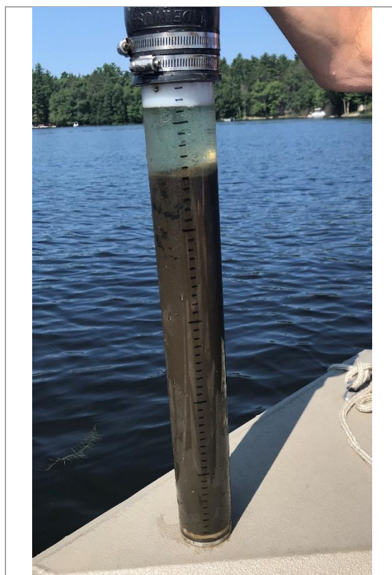
Photo 3.2-2. Photo of sediment core collected from Towanda Lake. Below 15 cm the color changed from dark brown to lighter brown which likely signifies when logging occurred.
