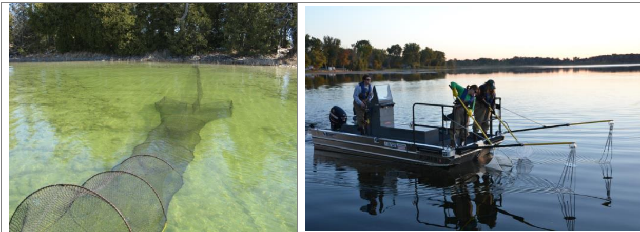
Photograph 4.2-1. Fyke net positioned in the littoral zone of a Wisconsin Lake (left) and an electroshocking boat (right).
