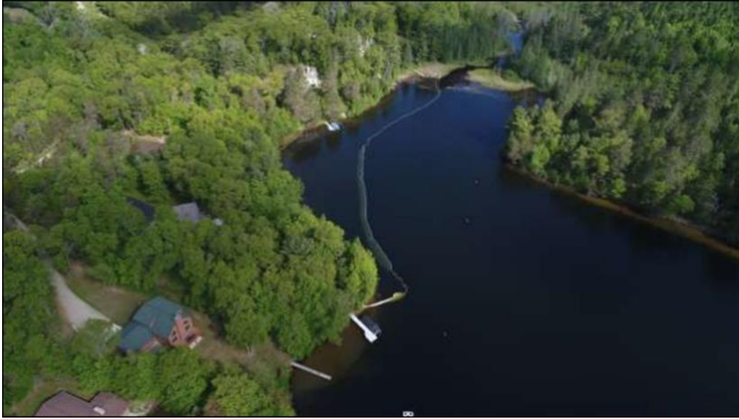
Figure 38: Limno-curtain installed on Thunder Lake (photo from Marinette Co. LWCD)
