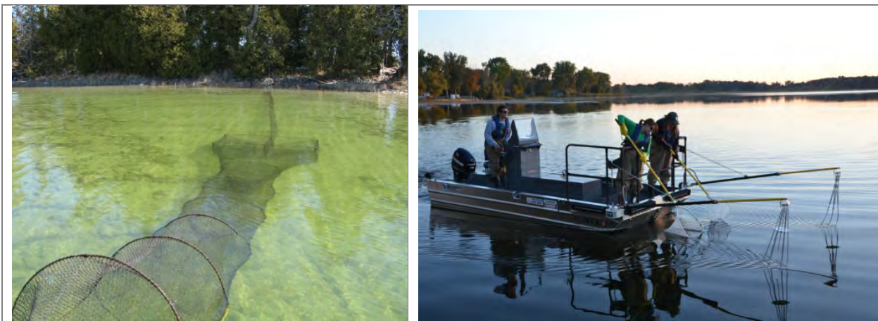
Photograph 8.7.6-1. Fyke net positioned in the littoral zone of a Wisconsin Lake (left) and an electroshocking boat (right).
