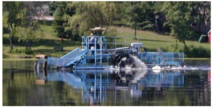
Photograph 3.5-3. Aquatic plant mechanical harvester.
