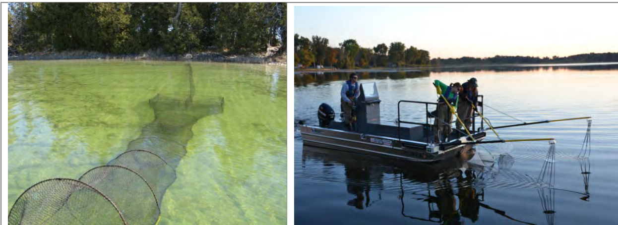
Photograph 8.5.6-1. Fyke net positioned in the littoral zone of a Wisconsin Lake (left) and an electroshocking boat (right).
