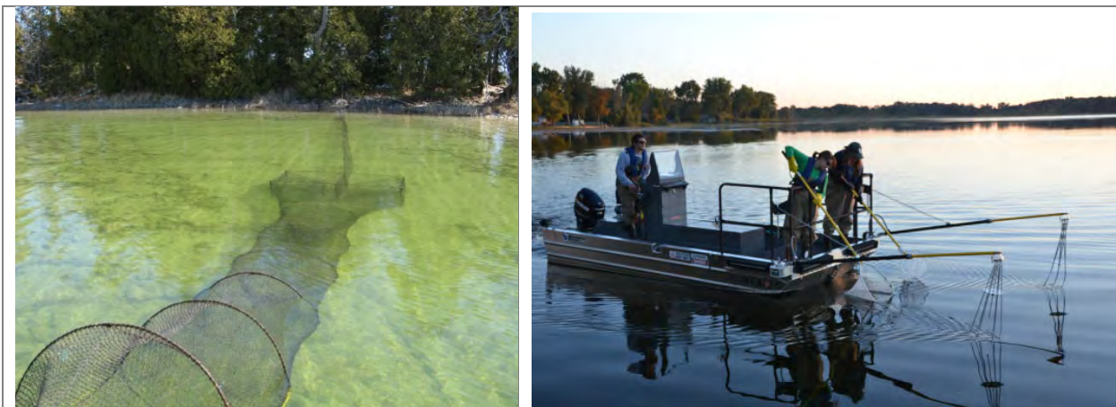
Photograph 8.6.6-1. Fyke net positioned in the littoral zone of a Wisconsin Lake (left) and an electroshocking boat (right).
