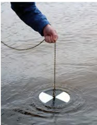
**Figure 23: Photo of Testing Water Clarity with Secchi Disk**
