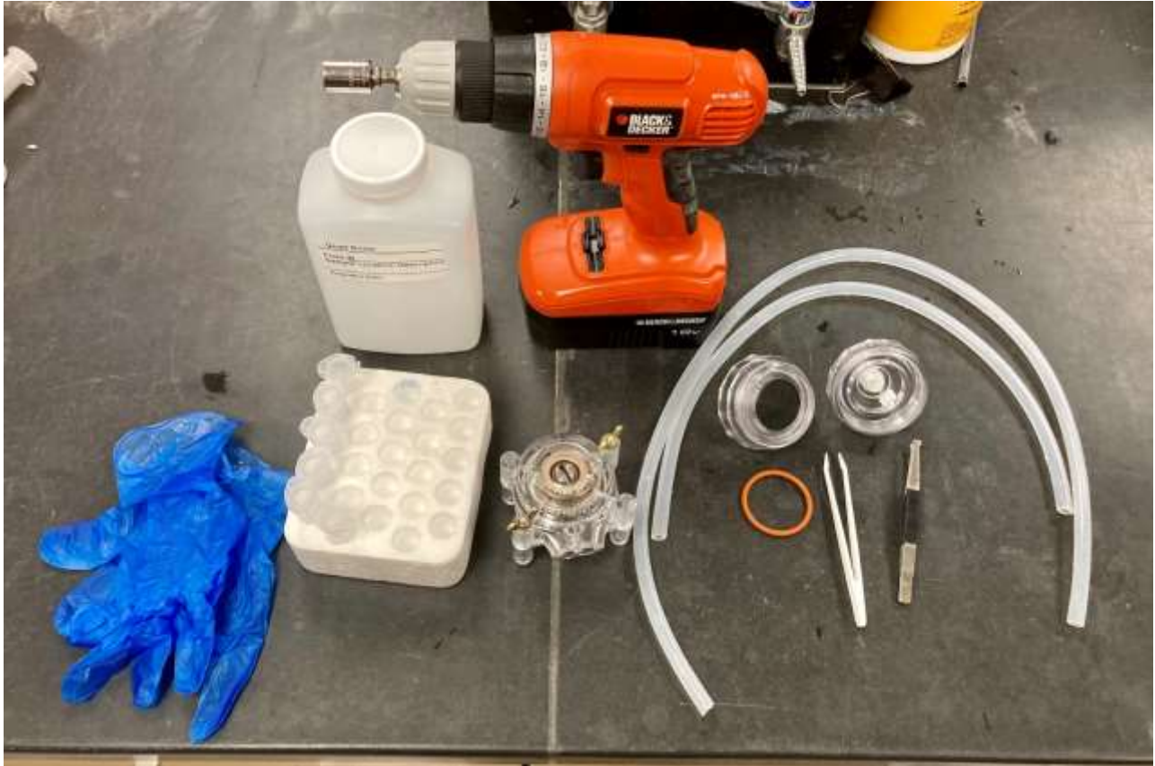
Figure 3 Sample bottles, peristaltic pump, tubing, filter tubes, tweezers, and gloves used for eDNA filtration.
