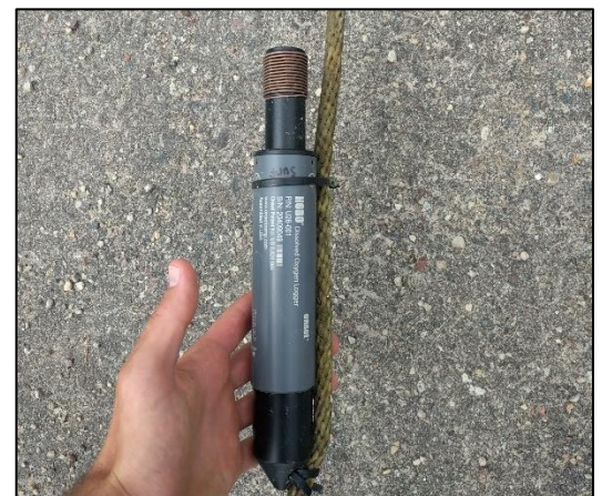
Figure 6. Dissolved oxygen logger installed vertically.
