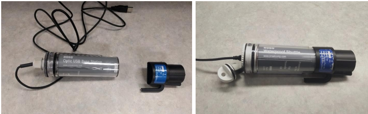
Figure 1. USB Base Station (left) and Waterproof Shuttle (right) with the coupler for Pro v2 temperature loggers.
