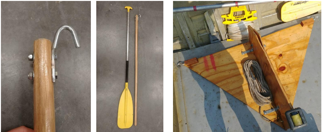
Figure 2. Potential tools for retrieving submerged equipment. The device on the left is a long pole with a hook. The device on the right (invented by Mica Kromrey) cruises beneath the water and intercepts the submerged equipment with one of the 2 hooks at the corners of the triangle. A SCUBA weight is used to partially sink the device.
