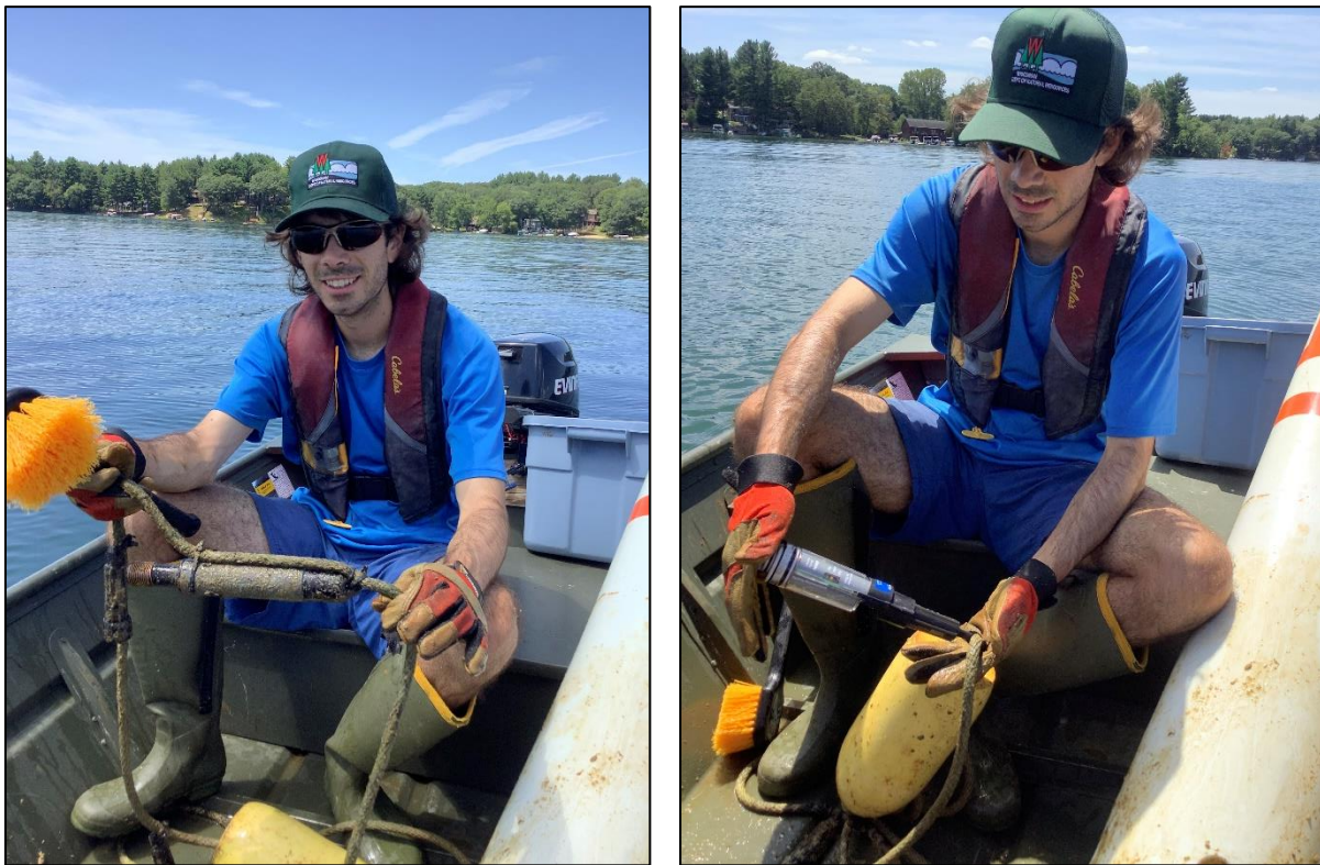
Figure 11. Dissolved oxygen logger with significant fouling is cleaned with a plastic brush (left). Temperature data is downloaded using the waterproof shuttle (right).
