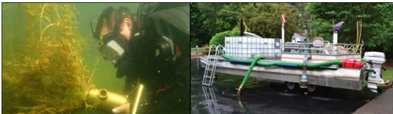
Figure 47: DASH – Feeding EWM into the underwater Suction Hose (Marinette Co.); and a sample DASH Pontoon Boat (Beaver Dam Lake Management District)
