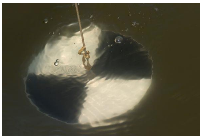
Figure 7: Black and white Secchi disk
