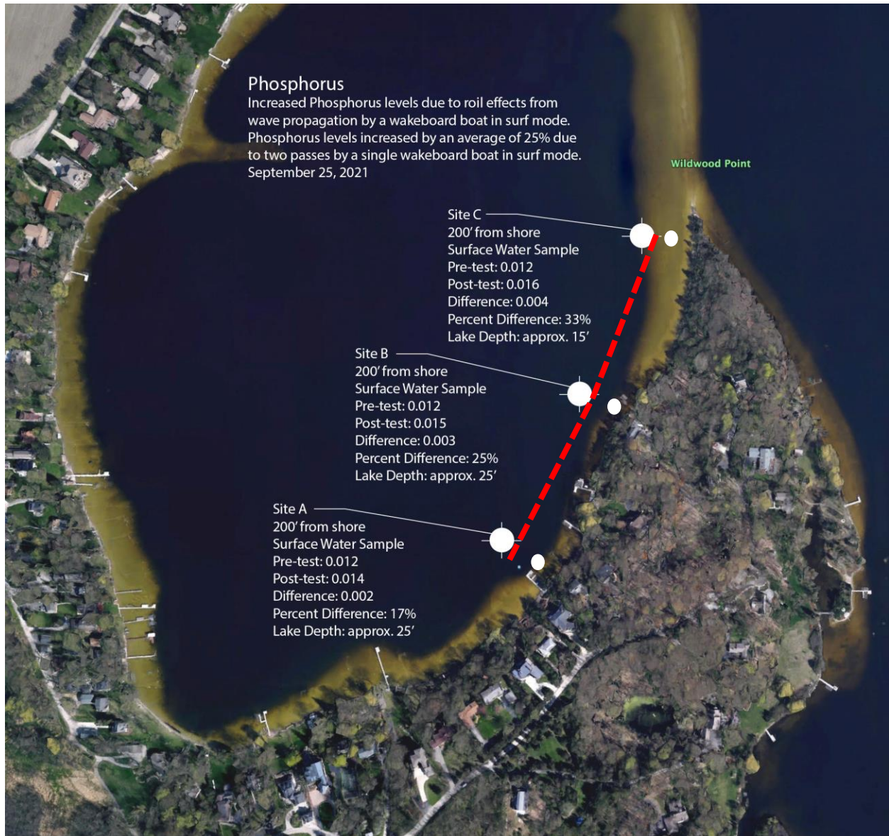
Figure 18: Course and Sampling Sites for Nutrient Load Differences (pre-post) from Wakeboard Boat in Surf Mode
