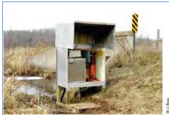
Figure 10 – Typical U.S. Geological Survey recording streamflow-gaging station with automatic water sampler for load determinations (Garn, Elder, & Robertson, 2003).
