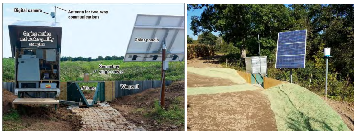
Figure 40: Example edge-of-field surface water monitoring station/system (left); actual Lake Redstone watershed edge-of-field monitoring station
