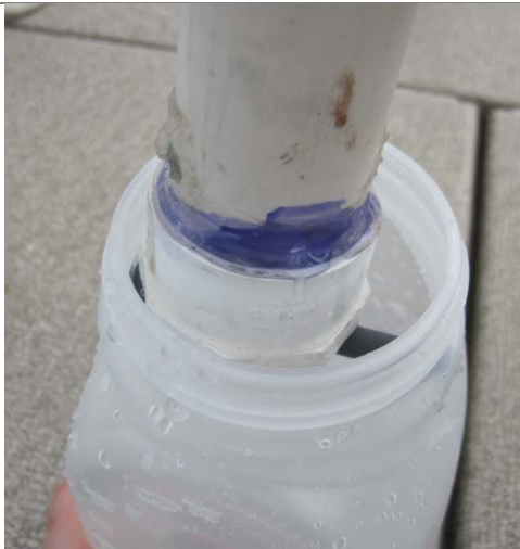
Photo 1. Six-Foot Integrated Sampler (top) & custom transfer bottle (bottom).
