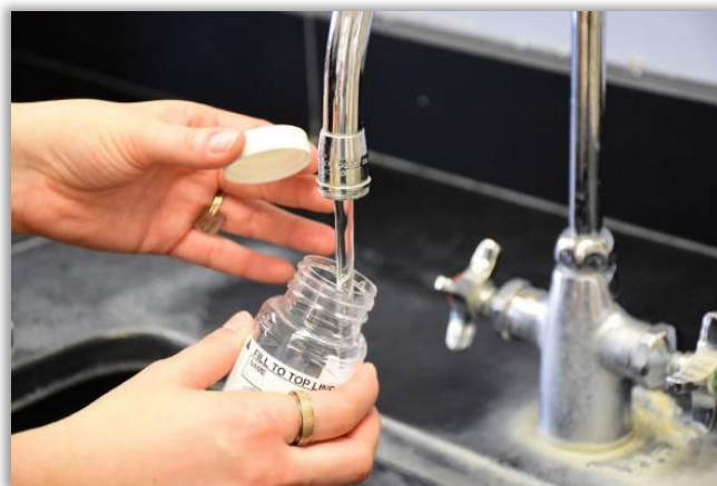
A State Lab of Hygiene employee demonstrates the proper procedure to collect a clean water sample (2020).
