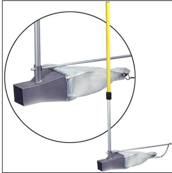
Figure 5 Photograph of “Helley-Smith” Stream Bed Load Sampler
