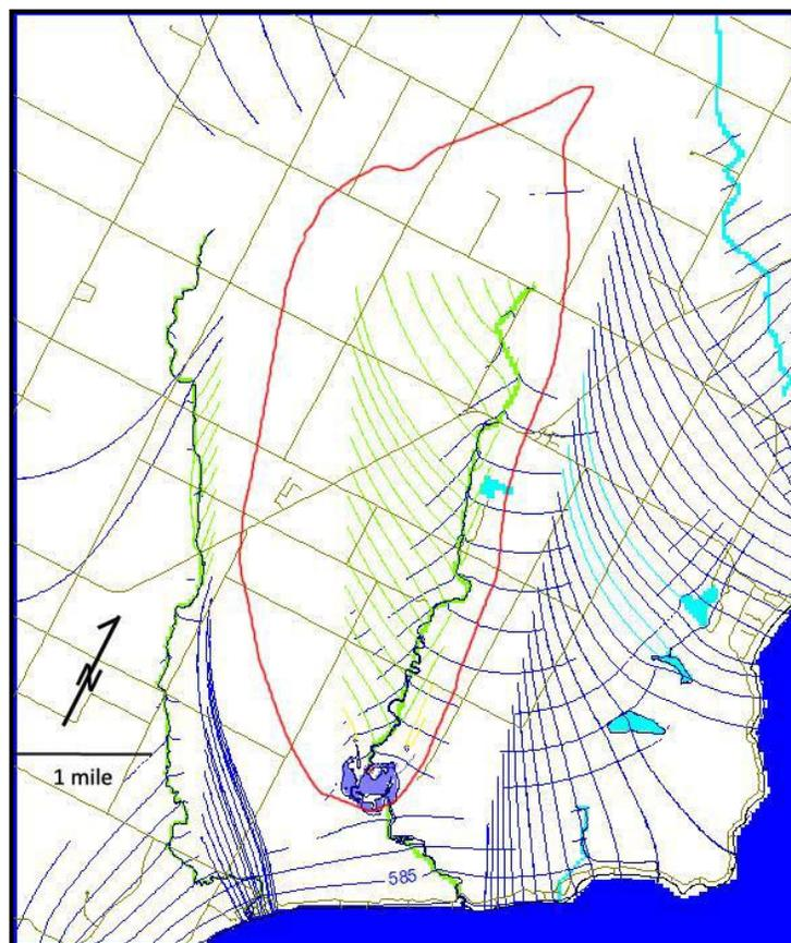
Figure 1.5 - Simulated groundwater flow with virtual particles as tracers.
