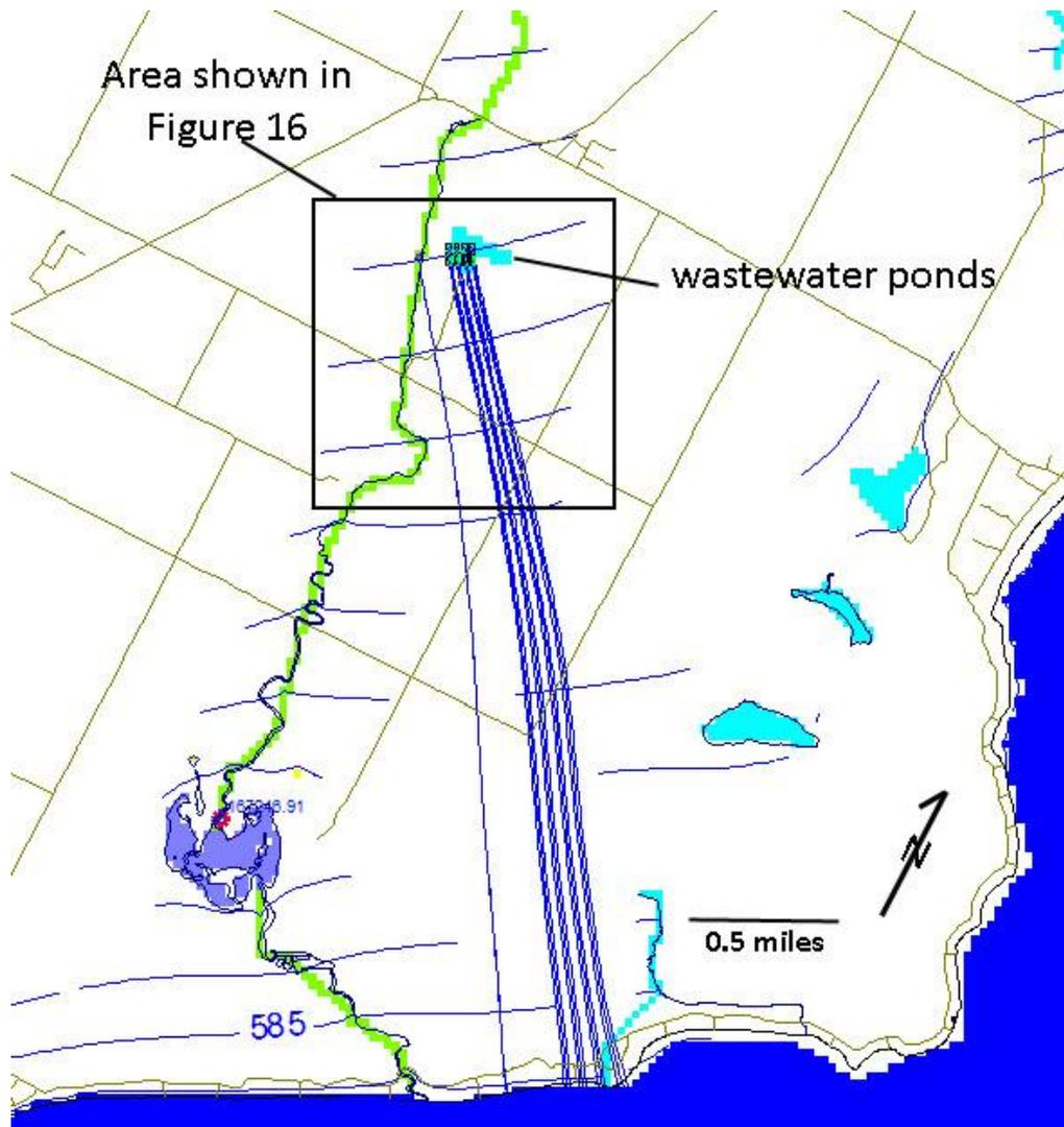
**Figure 17** Flow paths (blue) from the wastewater ponds and Geisel Creek under the dry season model with reduced recharge to simulate pond leakage when Geisel Creek is dry near the ponds.
