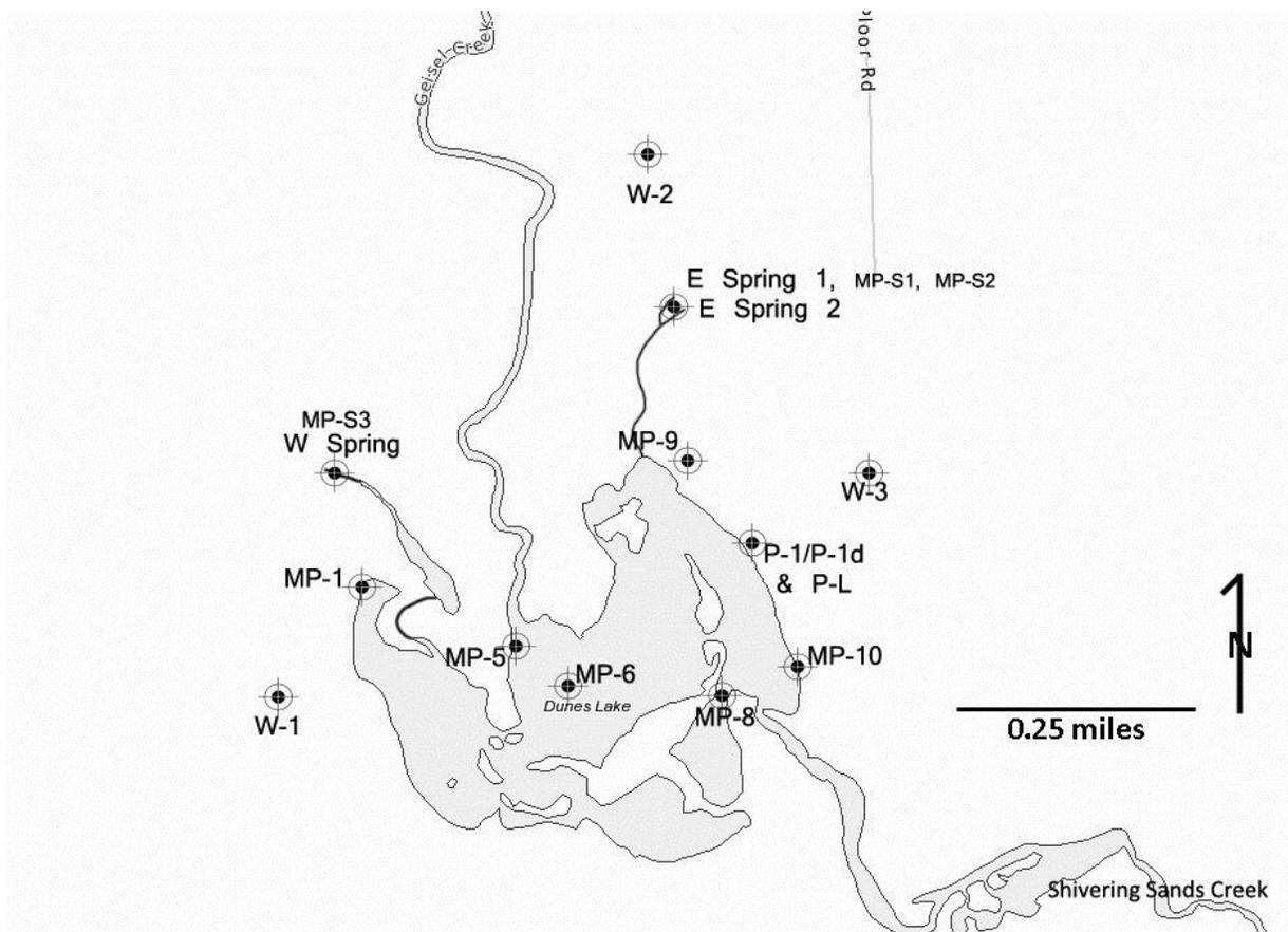
**Figure 3** Locations of installations for groundwater observations. Minipiezometers are designated with MP-, piezometers with P-, and bedrock wells with W-.
