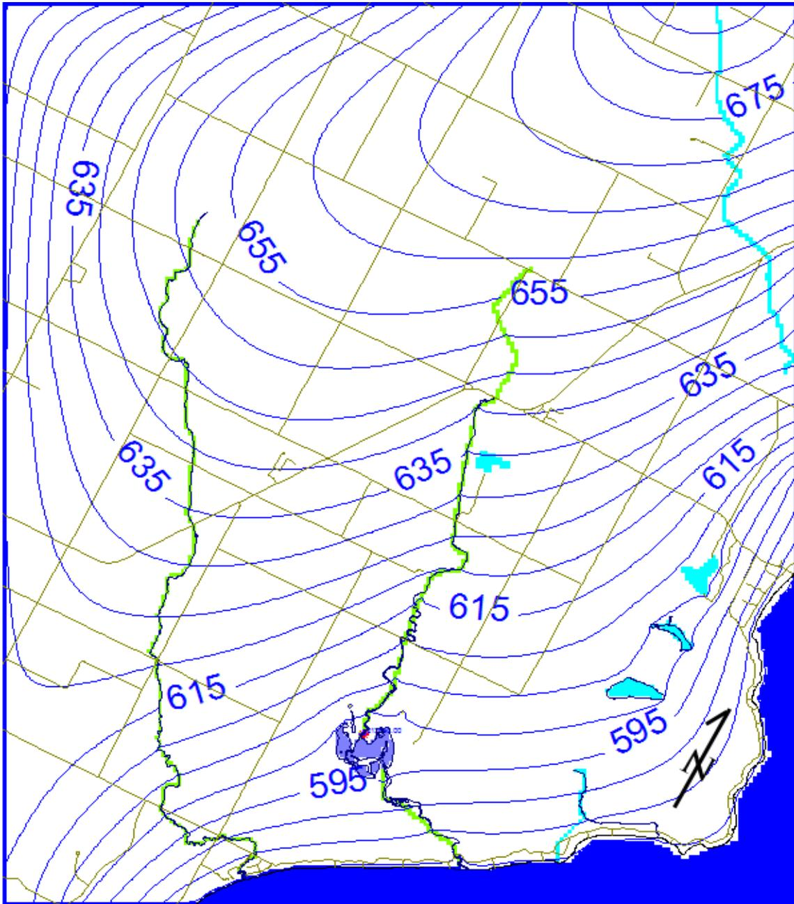
Figure 4.2 - Water table in dry season model. Contour interval is 5 ft.
