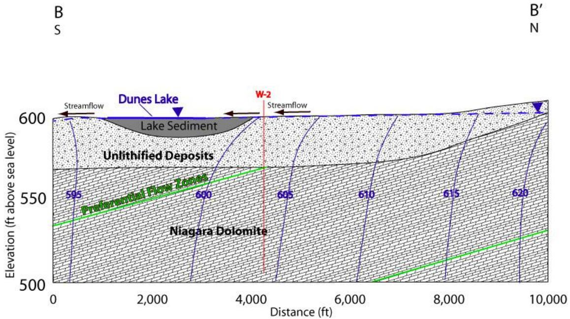
**Figure 12** Cross section through Dunes Lake along line B-B' in Figure 13 showing model results. Equipotential lines are shown with head in ft above sea level. Vertical exaggeration is 33x. While important to the bulk properties of the aquifer, the effect of individual preferential flow zones on flow paths near the lake is uncertain.
