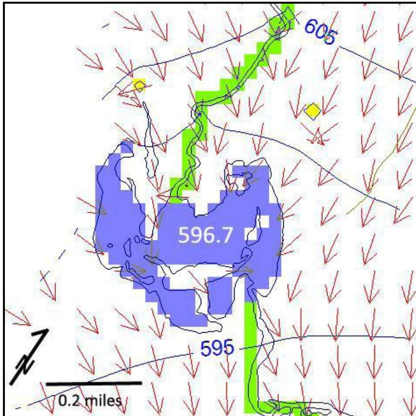
Figure 4.4 - Detail of groundwater flow around Dunes Lake, wet season model. Red arrows indicate direction of groundwater flow. Equipotential lines in layer 1 are shown with head in ft. above sea level.
