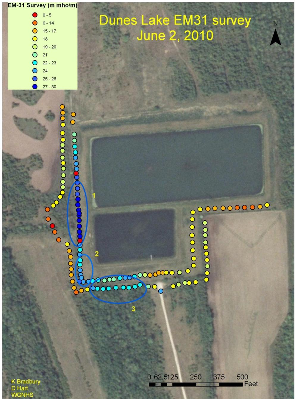
**Figure 8** Results of electrical resistivity survey around wastewater treatment ponds (courtesy of WGNHS 2010). Dark blue dots indicate measurements of high conductivity, which may be attributable to pond leakage.
