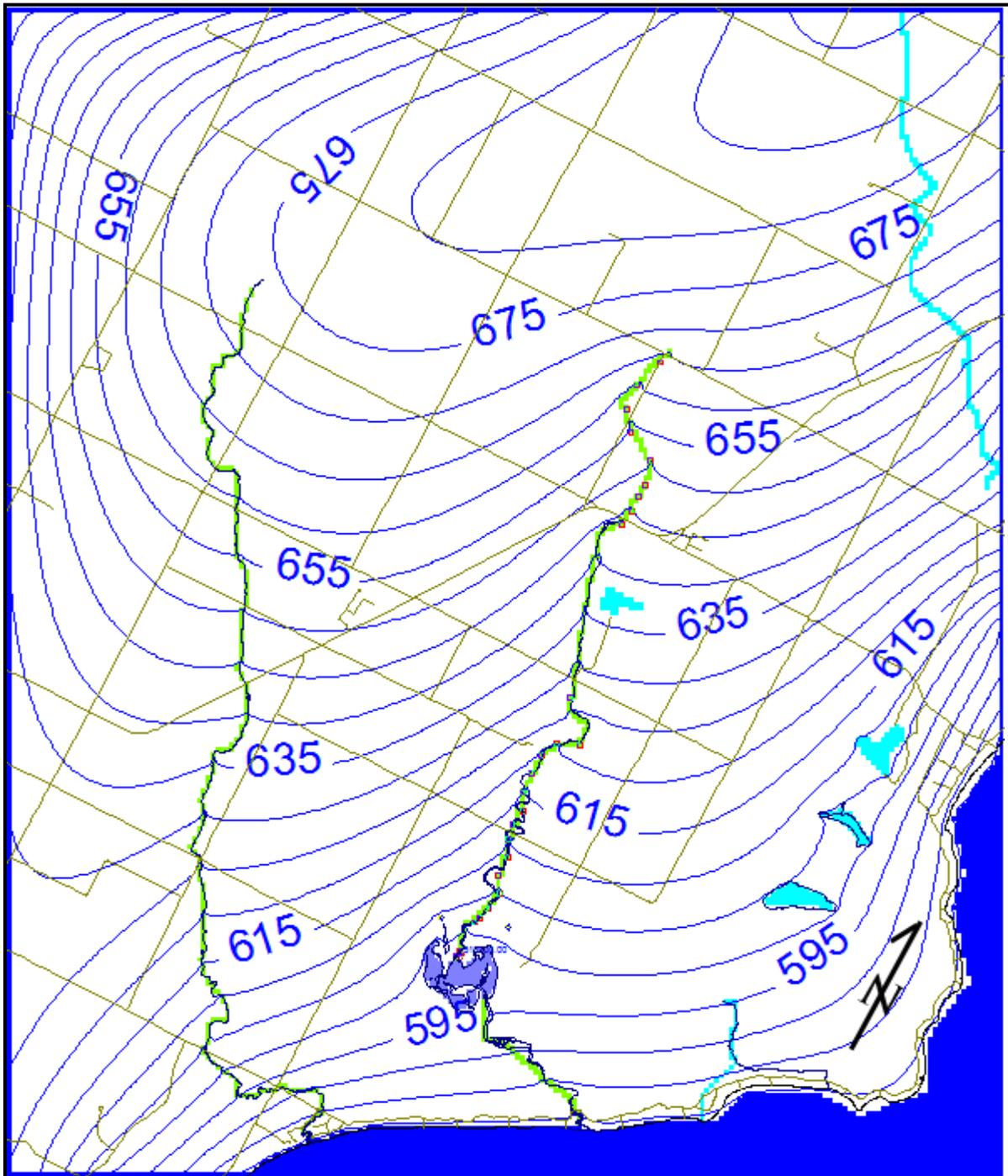
Figure 4.3 -Water table in wet season model. Contour interval is 5 ft. Note increased focusing of flow into Geisel Creek.
