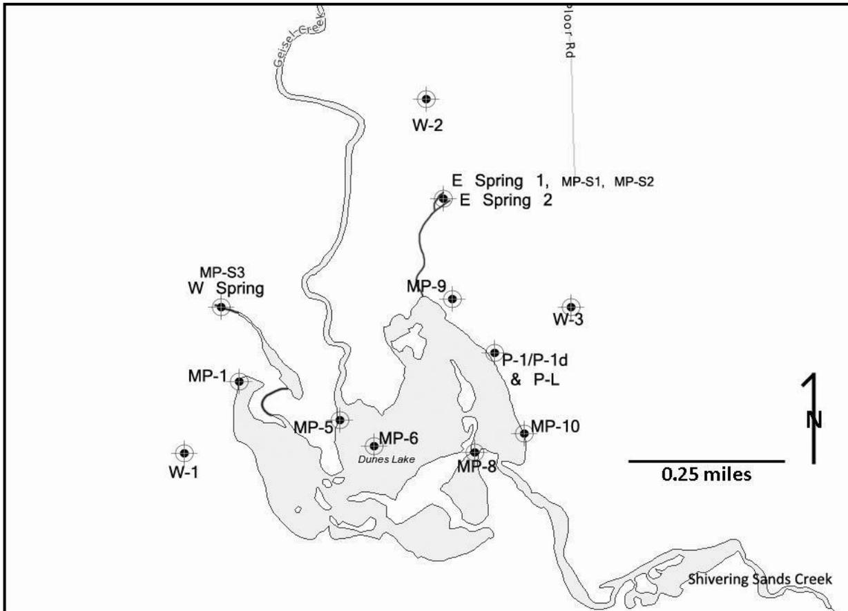
Figure 3.3 - Locations of minipiezometers (MP), and bedrock wells (W)
