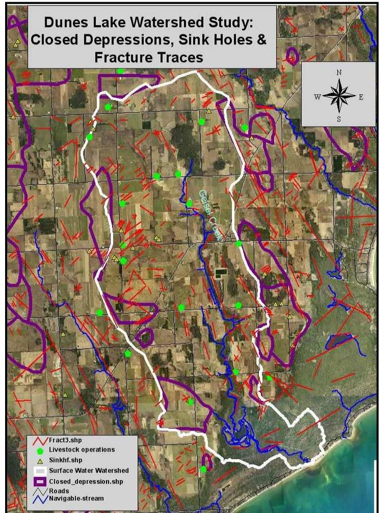
Figure 2.1 - Map showing closed Depressions, Sink Holes & Fracture traces within the Dunes Lake Watershed.
