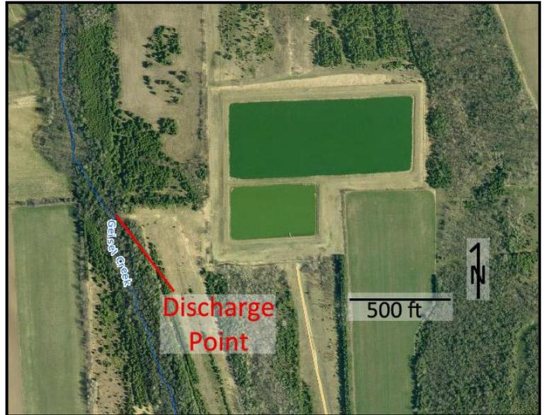
Figure 1.3 - Aerial Image of Wastewater Treatment ponds showing discharge point to Geisel Creek.
