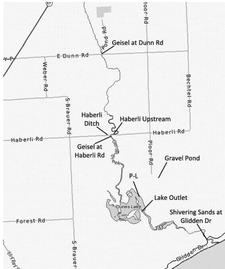
**Figure 5** Additional sampling locations. Haberli Ditch is a small stream flowing along Haberli Rd. into Geisel Creek. Gravel Pond is a small pond filling a former gravel pit. P-L is a piezometer installed at the edge of Dunes Lake screened along the upper 4 ft of lake sediment.
