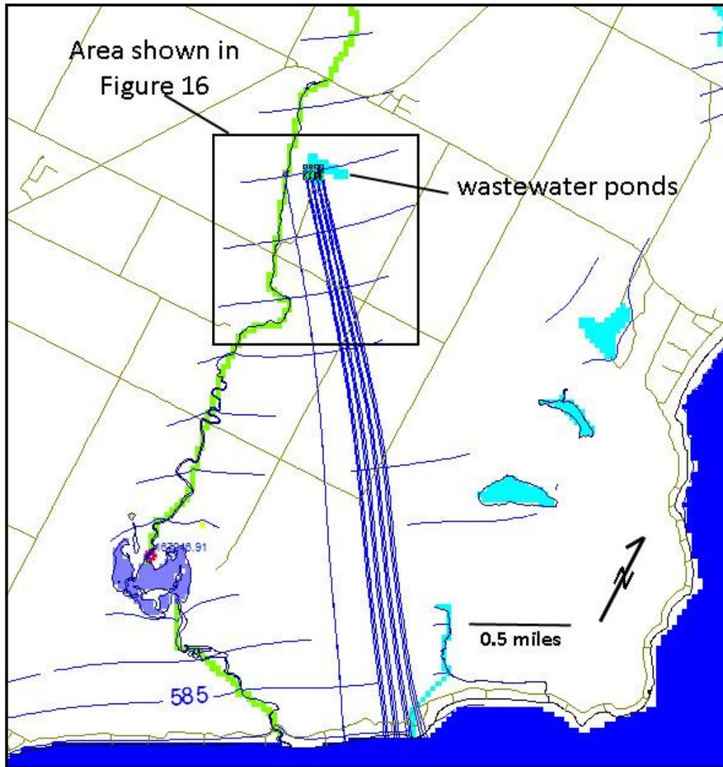
Figure 2.5 - Flow paths (blue) from the wastewater ponds and Geisel Creek under the dry season model with reduced recharge to simulate pond leakage when Geisel Creek is dry near the ponds.
