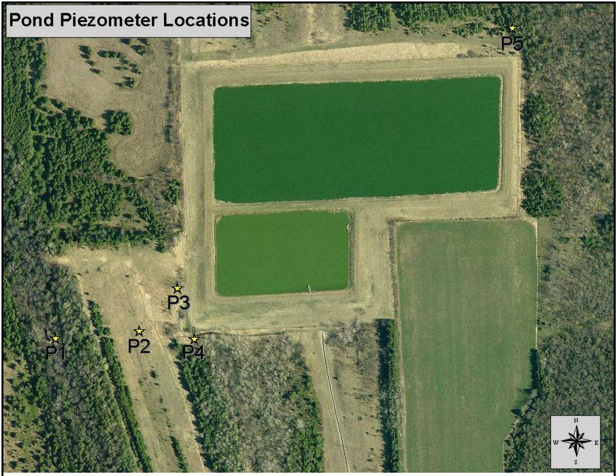
Figure 3.2 - Locations of piezometers around wastewater treatment ponds (Sevastopol Sanitary District No. 1)
