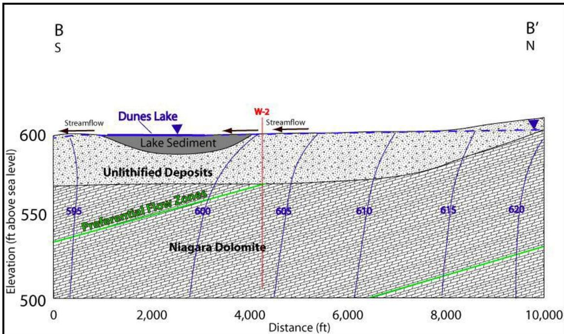
Figure 4.6 - Cross section through Dunes Lake along line B-B' in Figure 13 showing model results.
