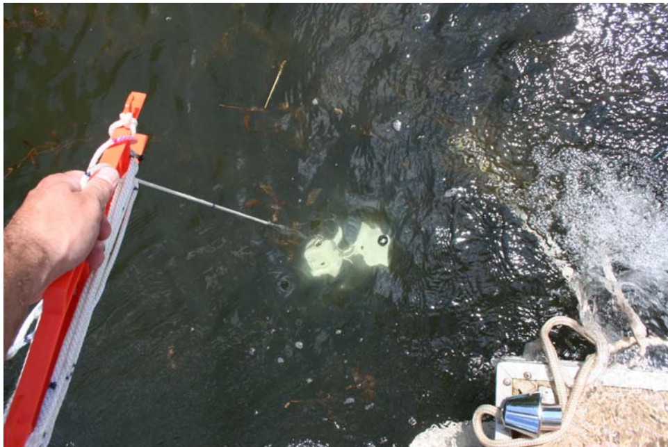
Figure 6. Secchi Disk reading off bow of HCS while in operation.
