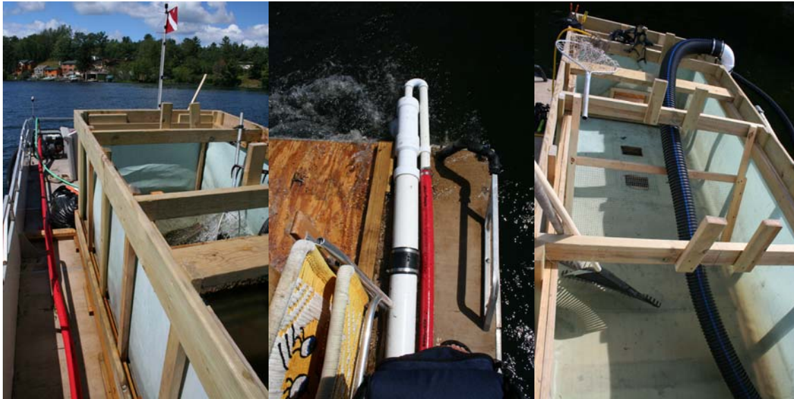
Figure 2. HCS pumps, hoses, and catch basin.
