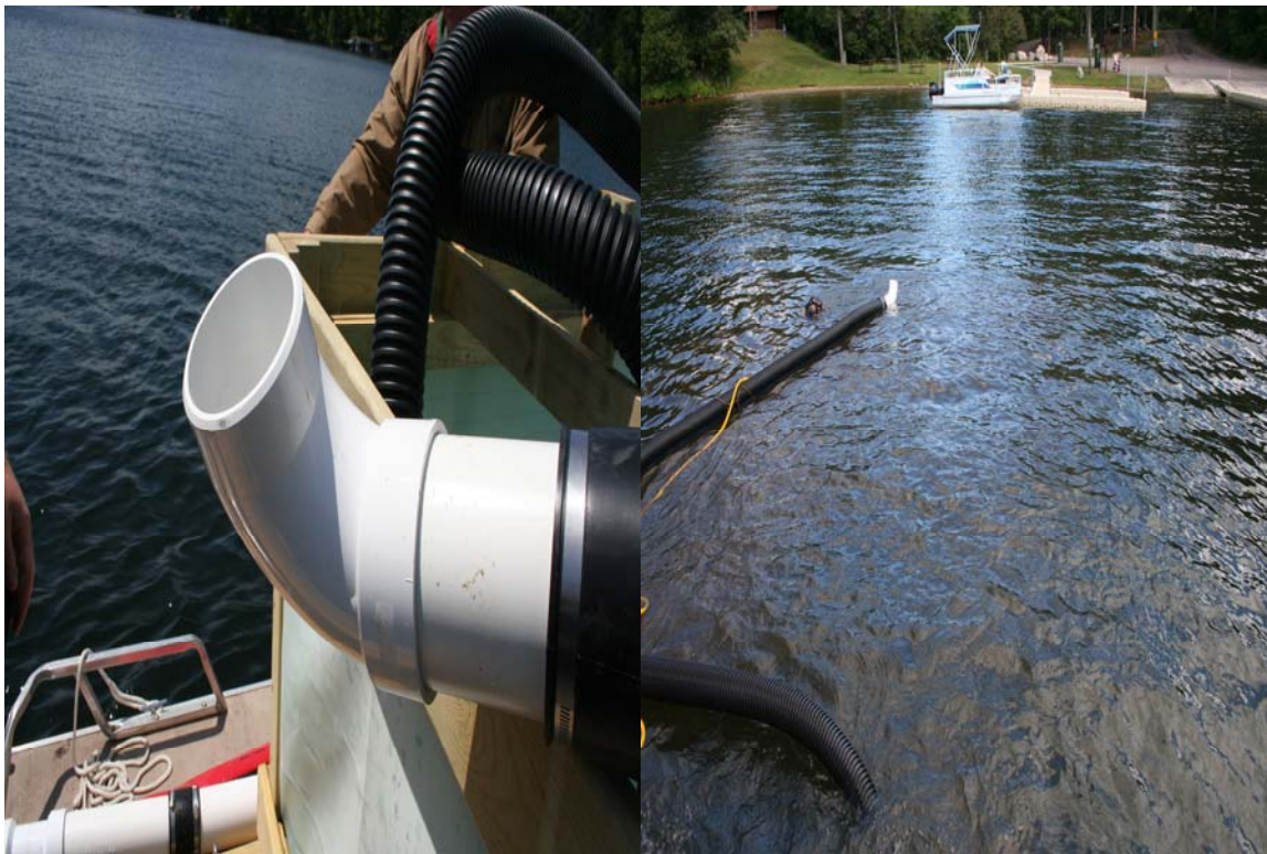
Figure 1. The upward facing flange (left) on the end of the HSC 8” diameter hose (right).
