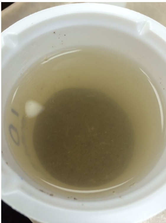
Photo 9. Settled Tox Site 1 elutriate over sediment sample with film on top.
