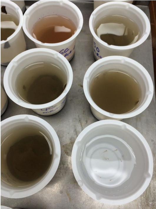
Photo 7. Acute P. promelas tests set up with organisms – orange colored sample on top left is synthetic sediment elutriate control, bottom right is lab culture water control. Note difficulty in seeing fish in some of the samples.
