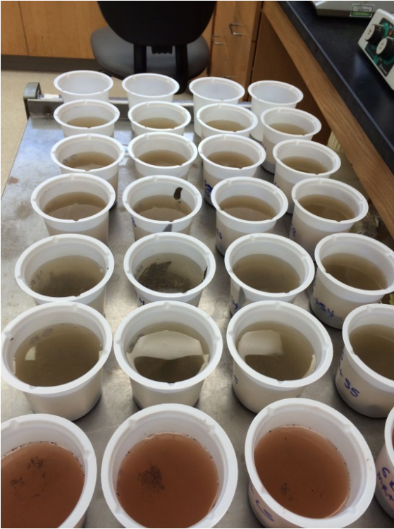
Photo 12. Sediment testing with Hyaella azteca .
