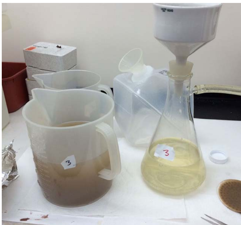
Photo 4. Filtering of elutriate from Tox Site 3.
