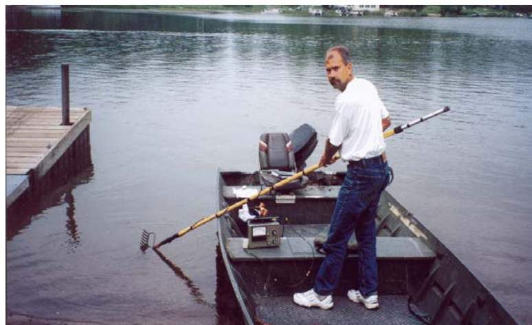
Figure 9. The conductivity survey consisted of attaching a conductivity probe to the end of a pole and moving around the lake in the shallow shoreline area. The conductivity meter recorded changes in conductivity.
