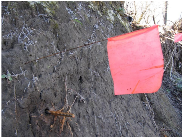
Figure 48. Erosion pin inserted into a streambank in Iowa. Photo Credit: Allamakee Soil and Water Conservation District, Iowa.
