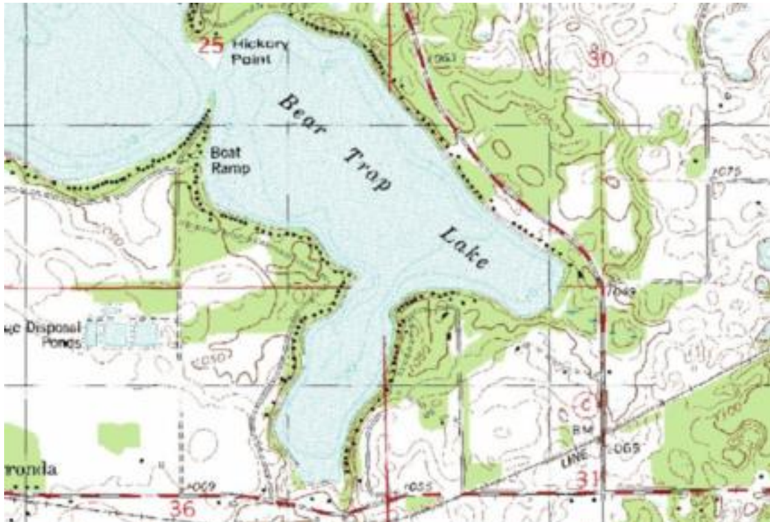
Figure 2: Topographical map of Bear Trap Lake. The east shore and the southeast point have steep elevation changes.
