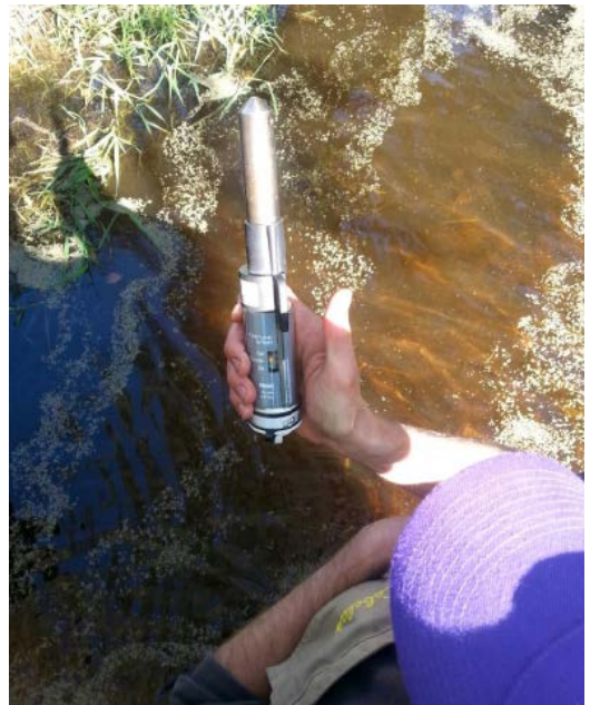
Pressure Transducer can be used to measure water levels in streams or wells.
