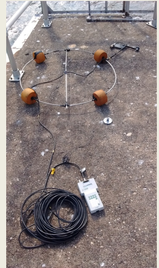
LI-COR sampling equipment used to measure 1 % of surface light.
