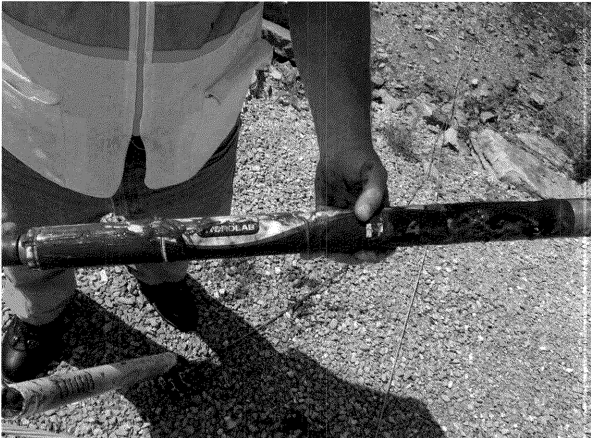
Photo No. 2 Example of sedimentation that occurred at Badger Downstream. Photo taken 6/29/15.
