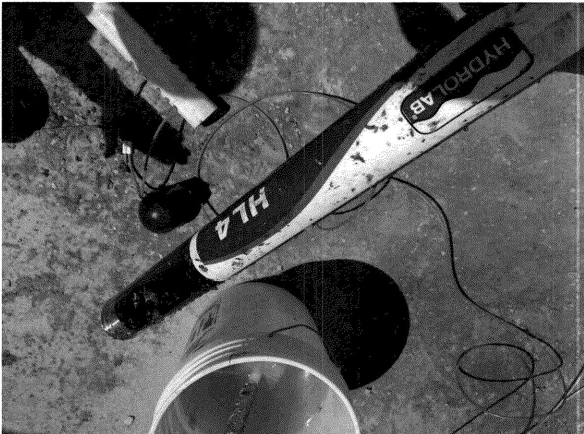
Photo No. 4 Example of mechanical problems that occurred due to aquatic organisms with hard shells becoming lodged in battery housing at Rapide Croche Downstream. Photo taken 7/28/15.
