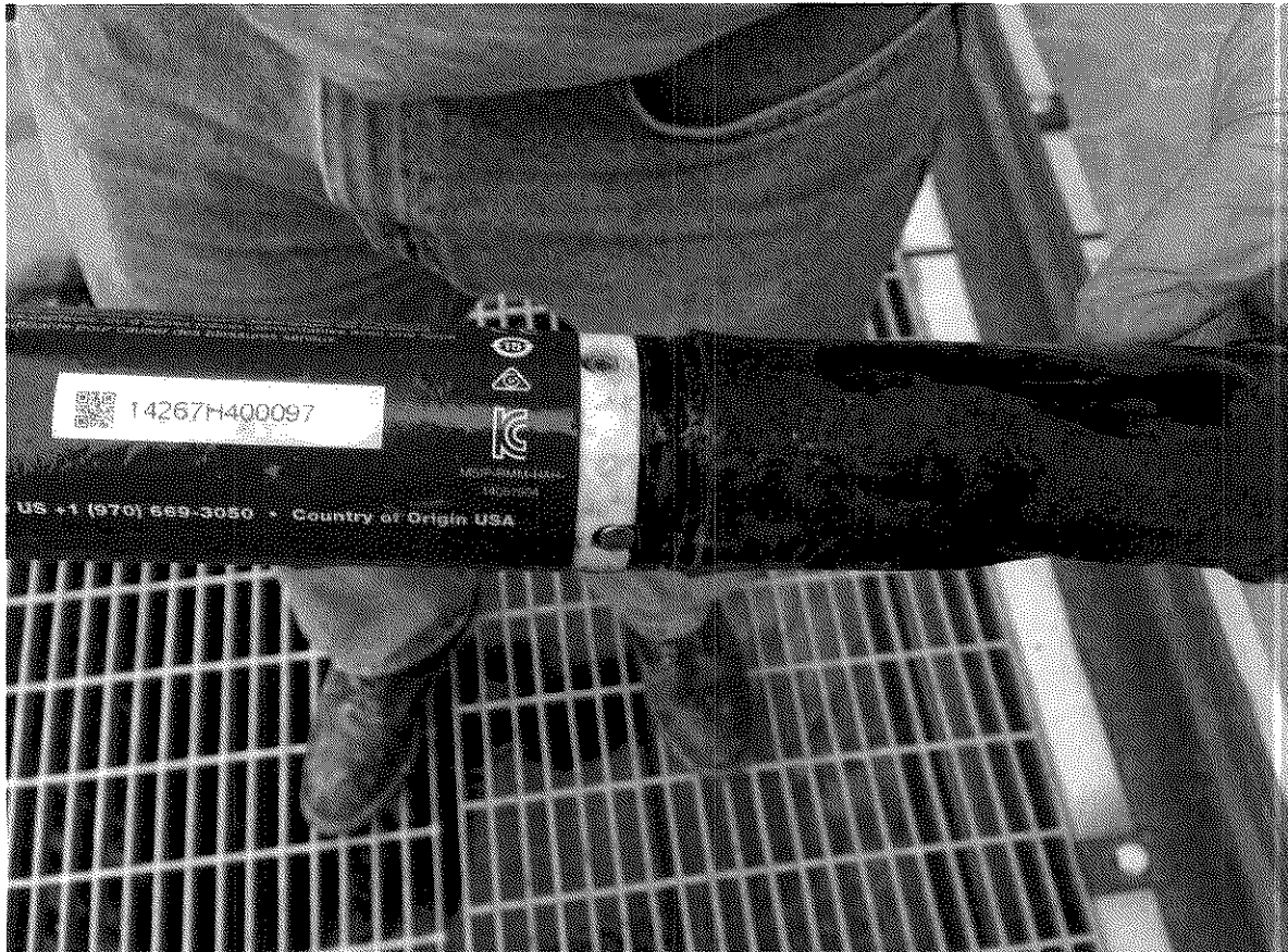
Photo No. 3 Example of biofouling that occurred at Rapide Croche Upstream. Photo taken 8/28/15.
