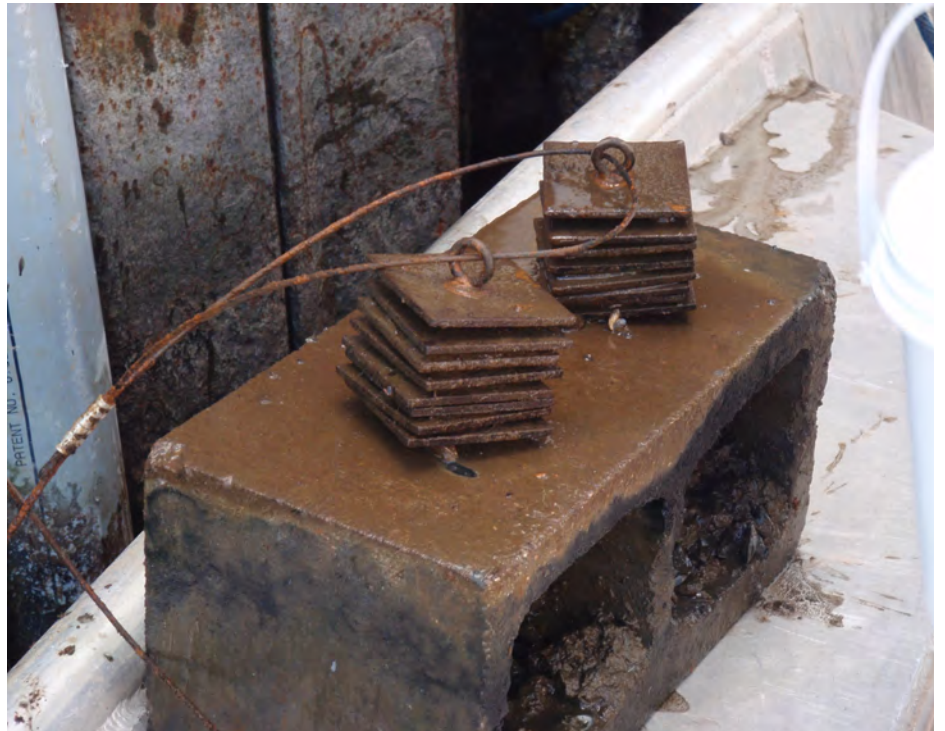
Figure 19. Hester-Dendy artificial substrate samplers retrieved for benthos community assessment.
