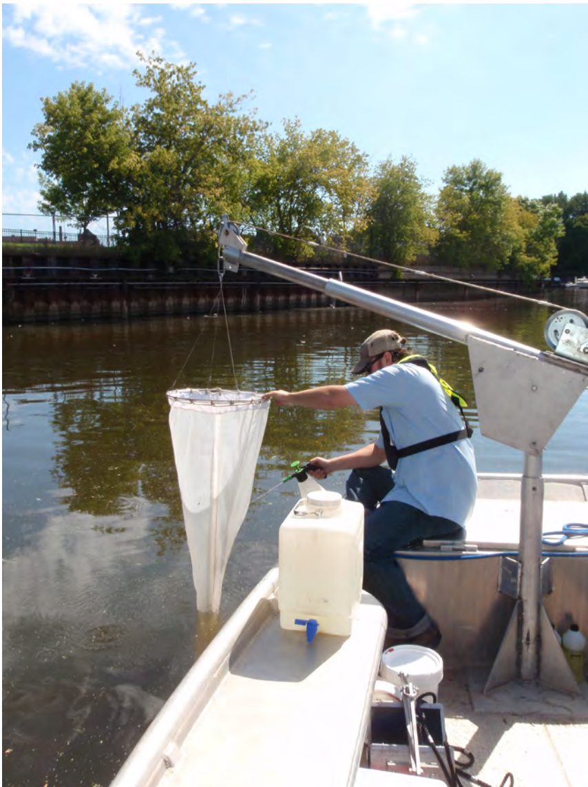
Figure 20. A plankton net being washed to collect a sample of zooplankton.
