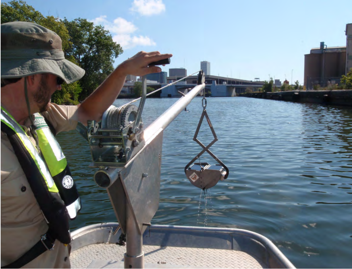
Figure 18. Ponar® dredge being retrieved with a grab for a benthos community sample.
